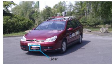
Fig. 1: The LIDAR mounted on the experimental vehicle.
