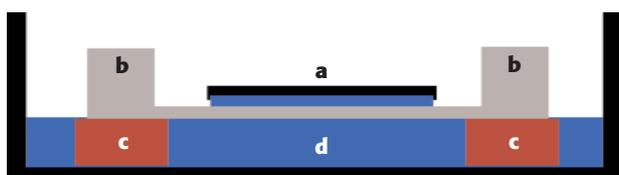
**7** Overall scheme of the treatment: The document (a) is placed on a silkscreen (b) supported by four blocks (c) at the corners. The tray is filled until the solution (d) reaches the screen. The weight of the document enables water to permeate through the mesh underneath the document only.
