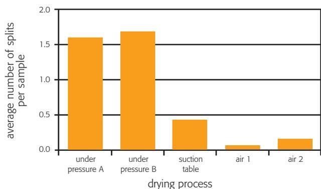
**6** Average number of splits appearing on the samples after drying. The drying processes are depicted in Tab 2.
