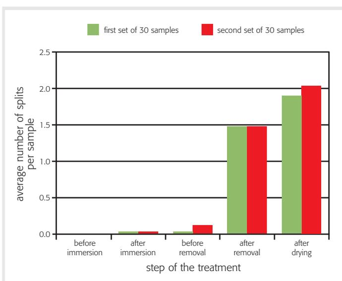
**4** Evaluation of the reproducibility of the experiment on two sets of 30 samples. During immersion and removal from the bath, the samples were manipulated with tweezers without any specific care (Tab 1: 'tweezers'). They were dried in open air. The removal of the samples from the bath was the most delicate action.
